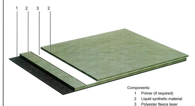
Applicable to the roof waterproofing "Triflex ProDetail":
